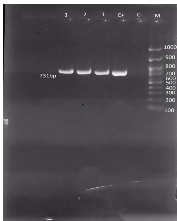
Figure 3. Gel electrophoresis showing the 731 bp PCR products from B. melitensis -specific primers (Br.m)
