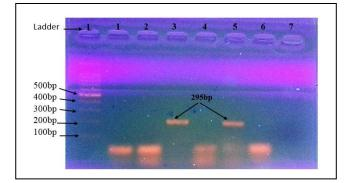
**Figure 2.** Agarose gel electrophoresis of amplified DNA of *H. controtus* by using primers (HcI-F, HcI-R) for amplifying the ITS-2 rDNA gene, Lane L, DNA ladder, Lanes 3,5 positive to 295 bp
