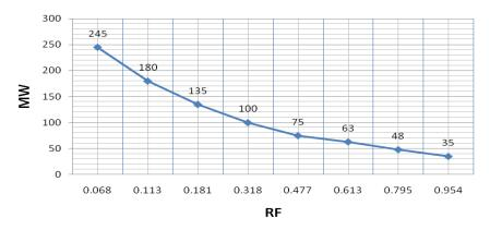
Figure 2. RF diagram against molecular weight
