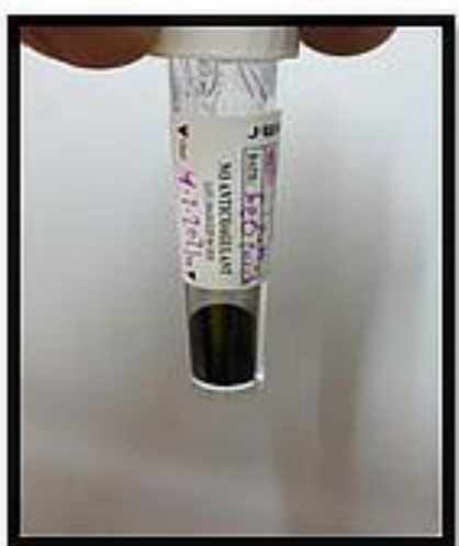
Figure 3. Dried magnetic nanoparticles isolated using an external magnetic field
