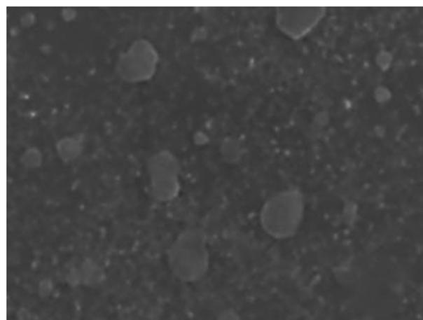
**Figure 4.** Crystalline clusters of AgNPs obtained by scanning electron microscopy (4000X)
