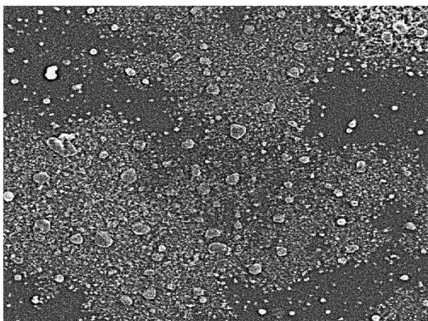
**Figure 3.** Crystalline clusters of AgNPs obtained by scanning electron microscopy (2000X)
