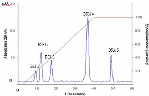
**Figure 3.** HPLC chromatography of BS31 obtained from DEAE-Sepharose chromatography. BS31 was applied on an HPLC C18 column which was equilibrated with solvent A (H<sub>2</sub>O, 0.1% TFA), and eluted with a concentration gradient of solvent B (acetonitrile, 0.1% TFA) from 0 to 100%, at a flow rate of 0.5 ml/min during 60 min.
