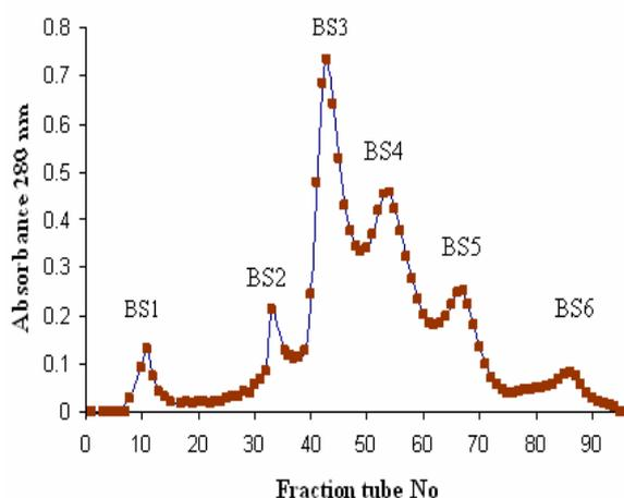
**Figure 1.** Sephadex G-50 chromatography of Iranian *Buthotus Schach* scorpion. Crude venom (135 mg) was applied to Sephadex G-50 column (3 × 150 cm) using buffer ammonium acetate 0.1 M and PH 7.5. Flow rate was 60 ml/hr and 9 ml fractions per tube were collected.
