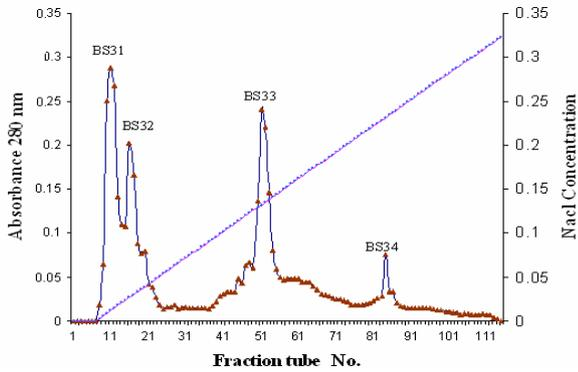
**Figure 2.** DEAE-Sepharose chromatography of BS3 obtained from Sephadex G-50. The pooled fractions from Figure 1 were applied to DEAE-Sepharose column (2.5 × 20 cm) equilibrated with 20 mM Tris±HCl buffer (pH 8.2). Proteins were eluted with a linear concentration gradient of NaCl from 0 to 0.5 M, and 5 ml fractions per tube were collected.
